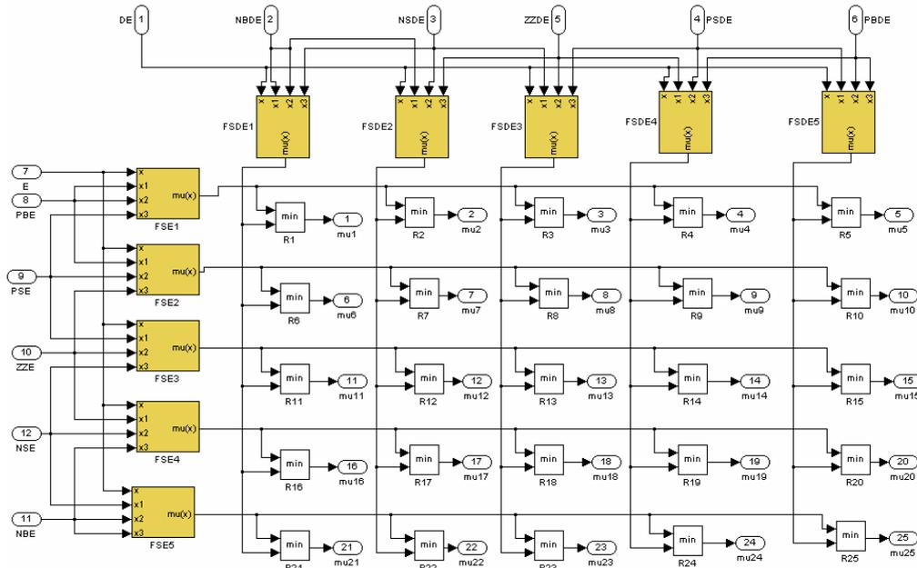
Fig. 4. The Simulink model of the Fuzzification process.
